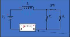
Initially, the meter reads same current as before the switch was closed.
