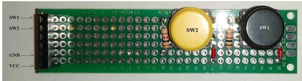
Connect SW1 to D2 (PD2), the SW2 to D3 (PD3) and Vcc (+5v) and ground (as shown above).
