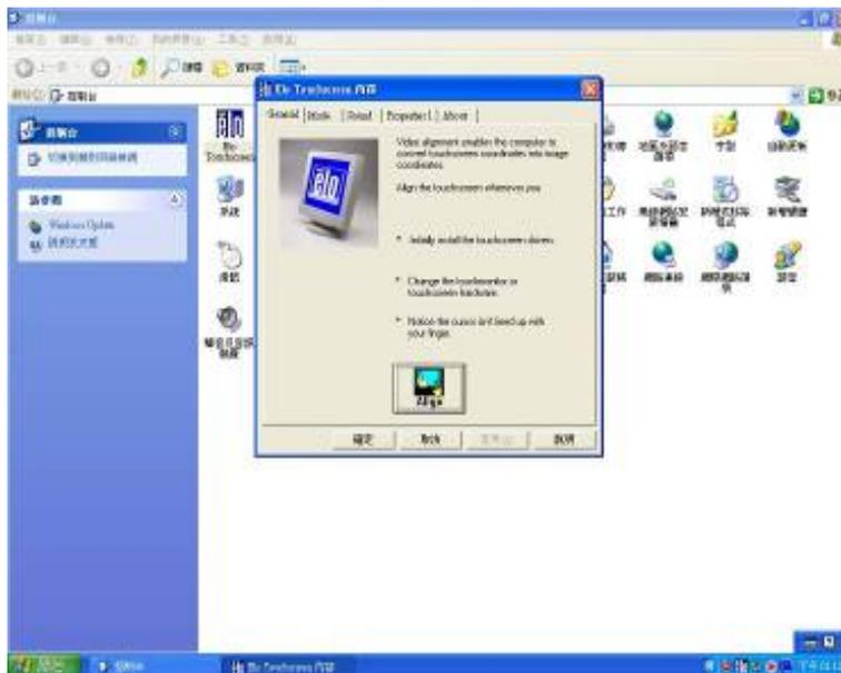
Step.3 Correct 4 point locations on screen with the Panel PC. Screen display as follows.
