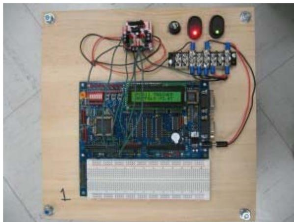
**Figure 6 – Suggested Component Mounting**
