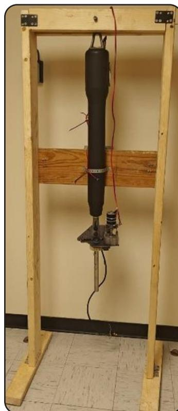
Figure 1: Prototype of the soil sampler
