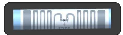
Figure 1. Ultra-High Frequency (UHF) RFID inlay tag
