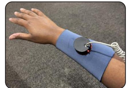
Figure 2: Sleeve, port, and transducer worn together. The sleeve provides better stability and ease of use than EXOGEN's strap, and the detachable port allows for easy cleaning of the fabric & plastic separately.
